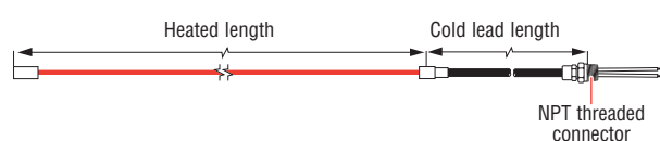
Design D: Dual conductor cable (32, 62 series only)
